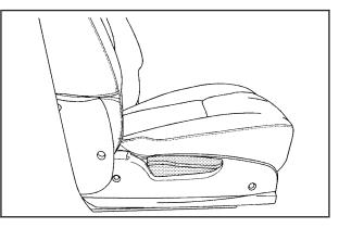
3. Lift up fully on the recliner lever, located on the outboard side of the seat, and fold the seatback forward until it disengages.
